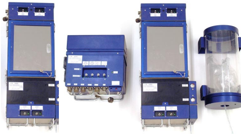
The LADA system, including two Vegetation modules, the Control Module and the Water Reservoir. The Vegetation module consists of three submodules, the light module, leaf chamber and root module.
