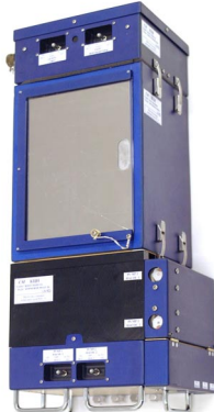
Details of the LADA Vegetation Module, including the light module, the vegetation chamber, and the root module. Each module has switches for manual or automatic operation.
