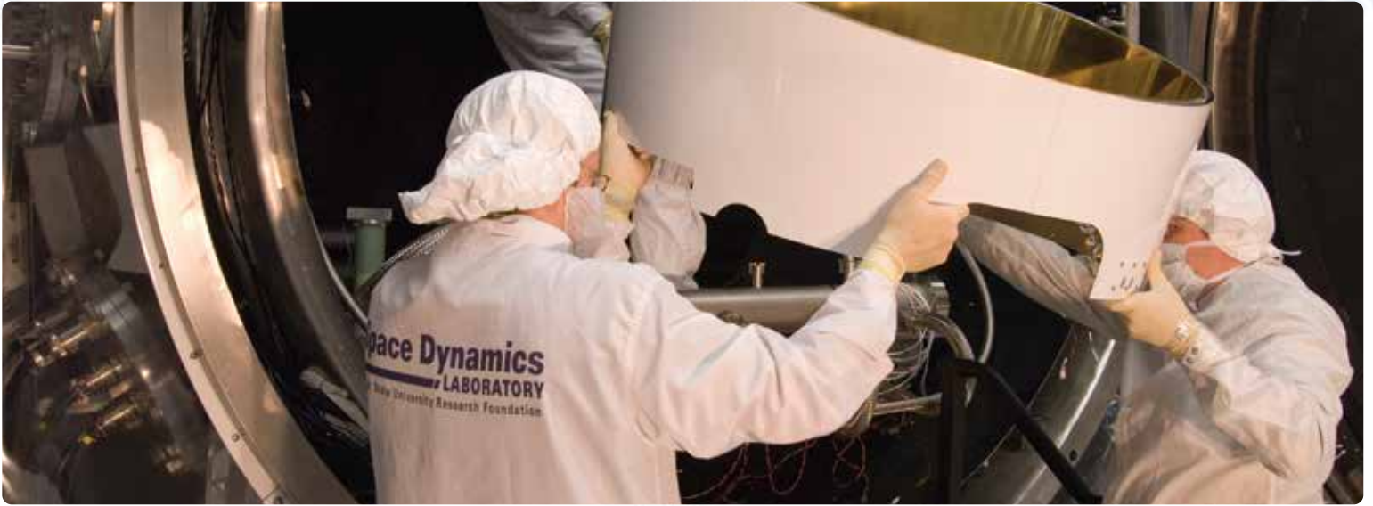
Placing the Wide-field Infrared Survey Explorer sun shade in the THOR chamber
