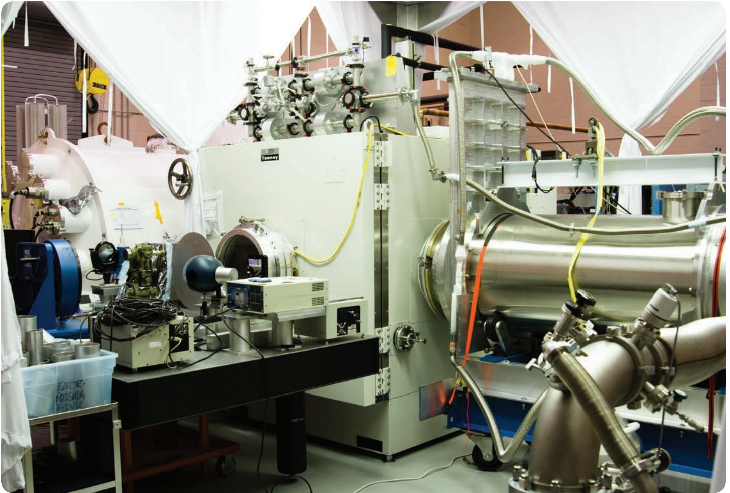
The Electro-optical Altitude Test Chamber interfaced with the MIC5 (left), HAES15 (right), and visible collimator/monochromator (front)
